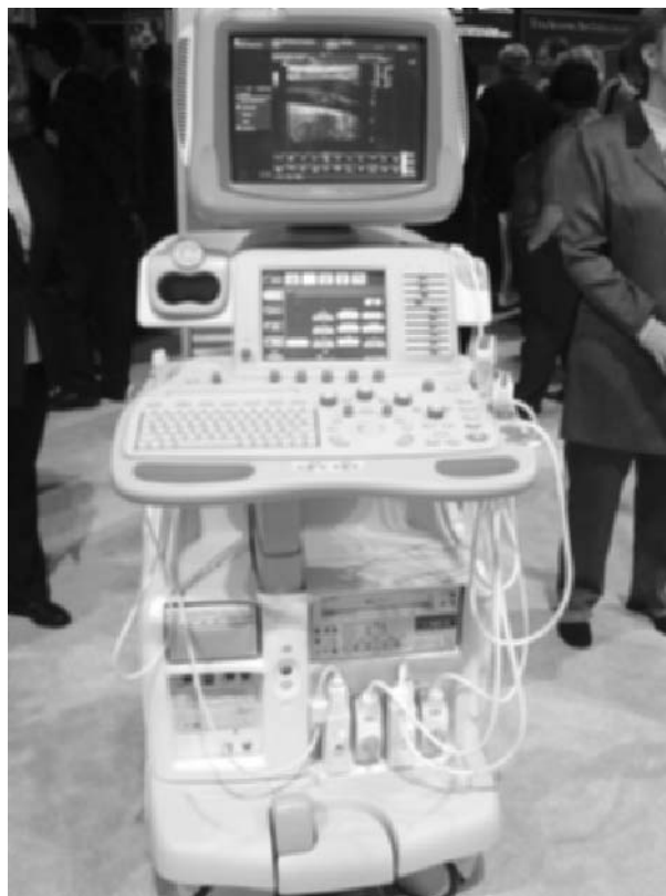
Figure 3.1 The basic components of an ultrasound machine are the monitor, the computer, and the probes.
