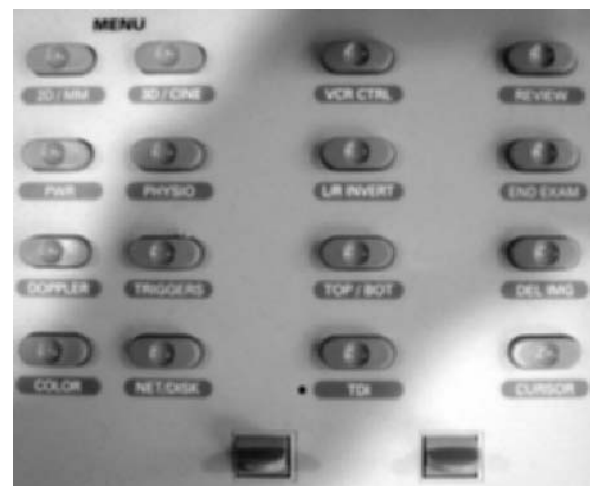
Figure 3.16 Special function keys – this includes the preset functions, dual display function, invert image, and other specialised functions such as extended field of view scanning (for example Siescape).
