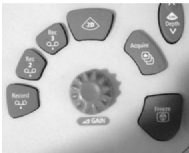
Figure 3.24 Cine, image store, and video recording facilities.
