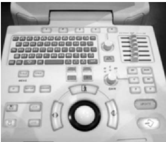
Figure 3.9 Key function controls – this includes the controls that are most commonly used, in particular the tracker ball, freeze, set and print buttons.
