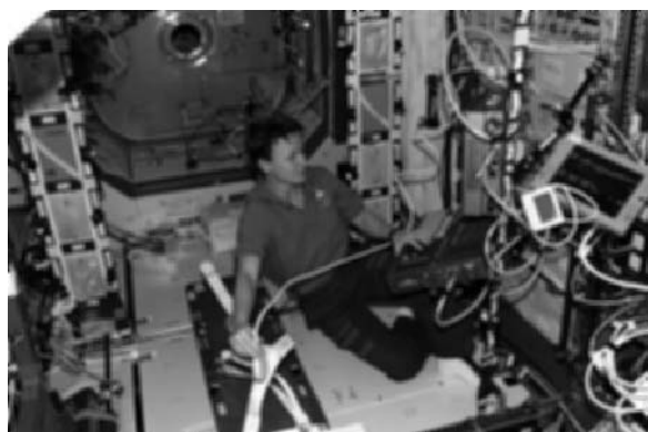
Figure 5.4 The NASA Human Research Facility Ultrasound Unit is shown onboard the International Space Station. The machine is a flight modified ATL 5000 ultrasound system and is equipped with a variety of probes.
