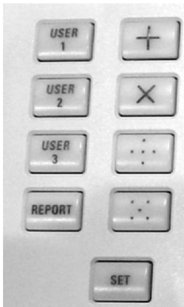
Figure 3.11 Measurement controls – these knobs are used in conjunction with the tracker ball to measure and annotate.
