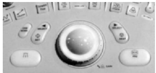
Figure 3.9 Key function controls – this includes the controls that are most commonly used, in particular the tracker ball, freeze, set and print buttons.
