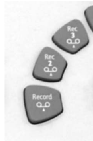
Figure 3.15 Peripheral controls – this relates to additional devices such as video, colour printer, optical disc storage, network imaging, or a paper printer.
